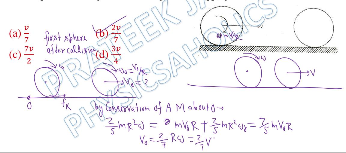
Q.11) A uniform solid sphere of radius r is rolling on a smooth horizontal surface with velocity v and angular velocity  $\omega$  (v =  $\omega$ r). The sphere collides with a sharp edge on the wall as shown in figure. The coefficient of friction between the sphere and the edge  $\mu$ =1/5. Just after the collision the angular velocity of the sphere becomes equal to zero. The linear velocity of the surface just after the collision is equal to
